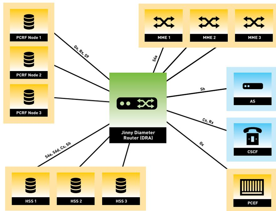
Figure 4: Signalling routing centralisation with a DRA
