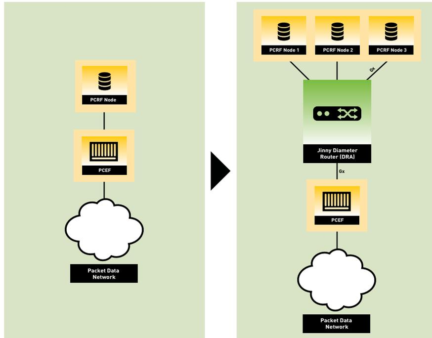
Figure 8: Scaling the PCRF using a DRA
