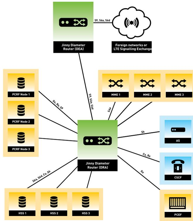
Figure 5: Signalling exchange between the home network and foreign networks using a DEA
