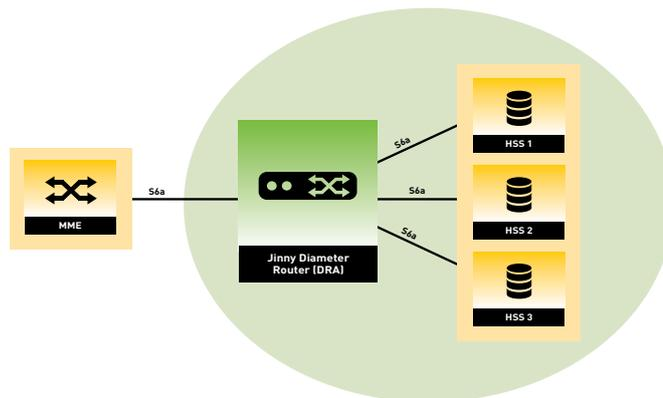
Figure 7: The DRA routes the Diameter messages from the MME to the correct HSS node using conditional routing
