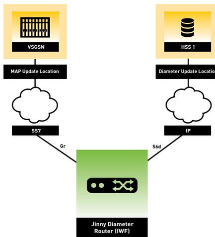
Figure 6: Signalling exchange between the home network and a foreign legacy network using the IWF part of the DEA
