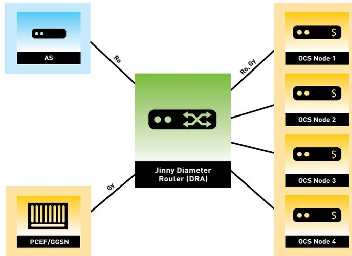
Figure 9: Distributing Diameter CCRs to a pool of OCS nodes
